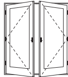
Active Panel Operating panel used most often
